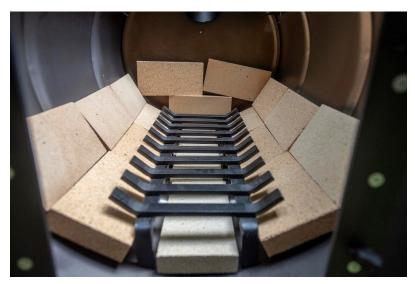
Unpack your *Sapling Fire Brick*. You are going to lay the eighteen fire brick in and up the sides of your *Sapling*. There is no magic to this, but you may note that the brick fit nicely in three rows of five brick each, with three bricks in the back of the barrel, as seen to the left. Note that the *Sapling Fire Brick* will fit in your barrel even if you have also chosen to purchase the *Sapling Fire Grate*, also shown.
