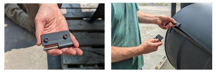
Slide the barrel hinge pieces on to the lid hinge pieces. (You may need or want to apply some WD-40 to the pin. You may need or want to use your mallet to help with the sliding.)
