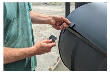
Slide the barrel hinge pieces on to the lid hinge pieces. (You may need or want to apply some WD-40 to the pin. You may need or want to use your mallet to help with the sliding.)
