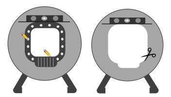
Place your unit on its feet on a level surface. Measure 16 inches up from the lowest part of the barrel lip. This will be the top edge of your door frame. Draw a level, horizontal line from the mark you just made.
