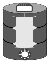
(Top view to show placement of flue pipe connection in relation to pan opening.)
