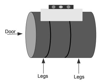
Dry fit the feet under the barrel and level the pan in the barrel opening.
