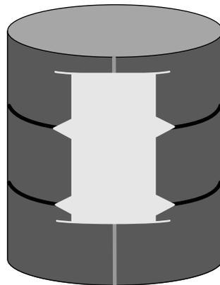
*Cut the barrel along the cutting lines, making extra triangular cuts on each rib.*
