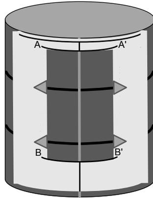
*Cut out and align the template with the barrel and mark cutting lines.*
