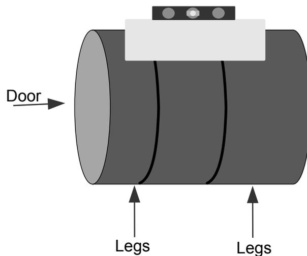
*Dry fit the feet under the barrel and level the pan in the barrel opening.*
