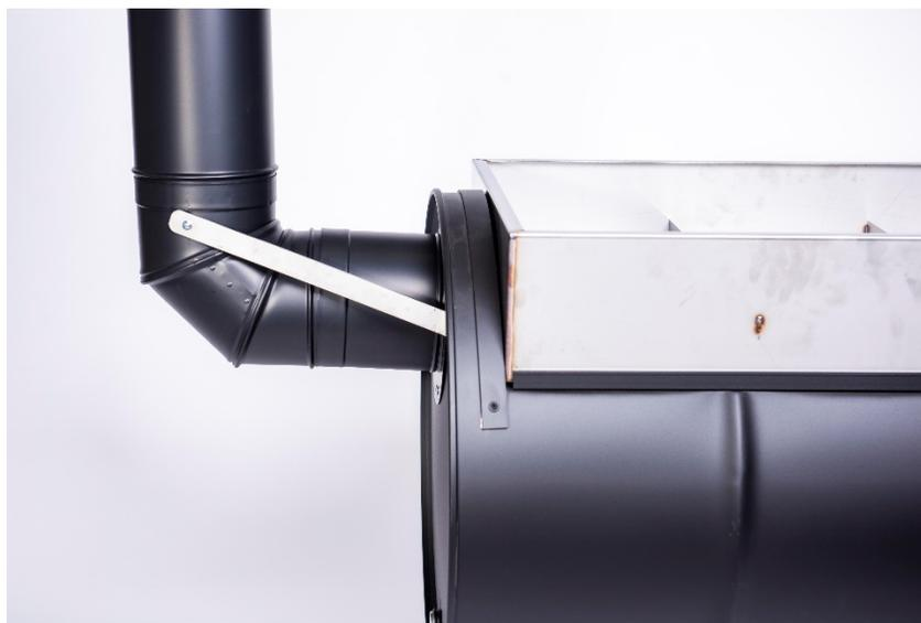
9. Fit a piece of flue pipe onto the elbow exit.
