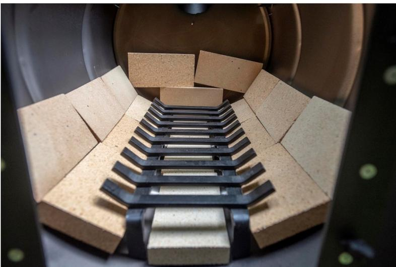
Now unpack your three boxes of *Sapling Fire Brick*. You are going to lay the brick in and up the sides of your *Sapling*. There is no magic to this, but you may note that the brick fit nicely with the fire grate when laid in five columns of three brick each, with three bricks in the back of the barrel. The *Sapling Fire Brick* holds the heat of the fire for the benefit of your boil, and also serves to protect the barrel from wear. *Sapling Fire Brick* will serve these functions whether
